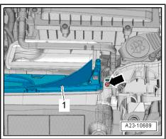
Lift off ventilator -1- (if fitted) with breather hose from the lock -arrow- on the battery tray -3-.
