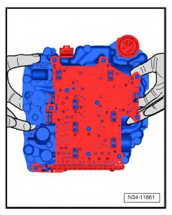
The sensors -arrows- must point upwards when the mechatronics is transported.
