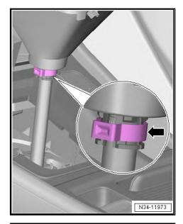
Detach the selector lever handle -1- together with the selector lever collar from the selector lever towards the top -arrow Aso that the lock button -2- is not pressed in.
