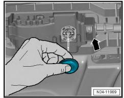
Detach the plug from the bottom part of the shift mechanism and take off the lock washer for the selector lever cable -arrow-.
