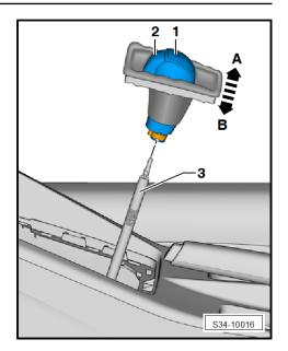
Carefully guide the release tool - T40203- fully into the selector lever handle -1- -arrow-.
