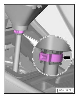
3.4.4 Removing and installing the cover with operating element for the gearshift mechanism - Octavia IV
