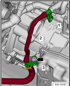
Remove screw -arrow- on coolant tube holder -3-, detach tube
