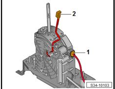
Disconnect plug connection for vehicle wiring harness to selector mechanism -1-.
