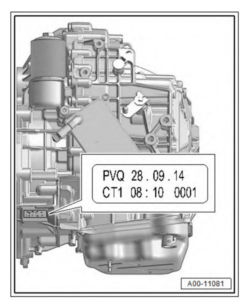
The gearbox identification characters are also printed on the gearbox.
