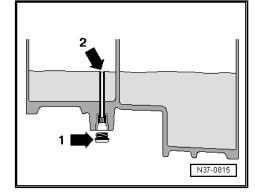
• Built up gear oil flows out of the overflow pipe -arrow 2-.
